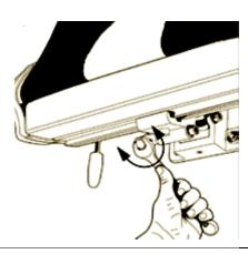
17) With spirit level check if front bar is levelled horizontally.
