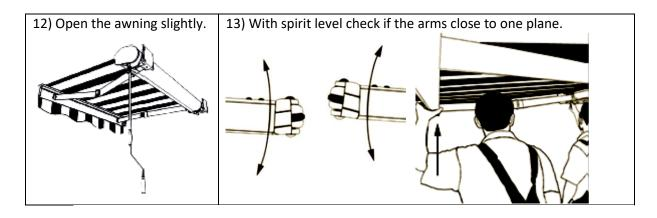
14) If necessary adjust the arm level by loosening or tightening the internal M5 screw in arm brackets.
