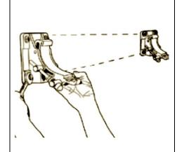
10) Slide the awning on wall brackets so that the construction is maximally pressed to the back (Note – before placing the awning verify the alignment of brackets – wall surface should be of the same thickness at installation spots).
